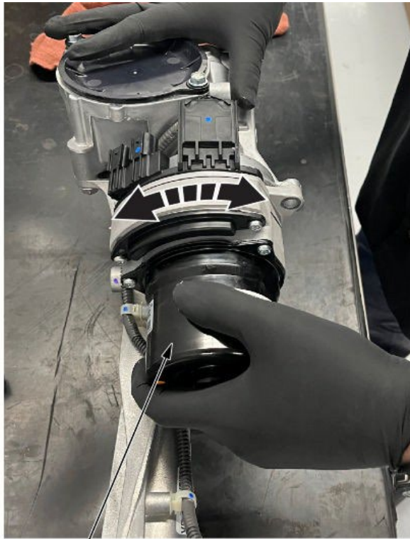
EPS MOTOR CONTROL UNIT Turn unit two or three times to the right and left (about 45 degrees).
