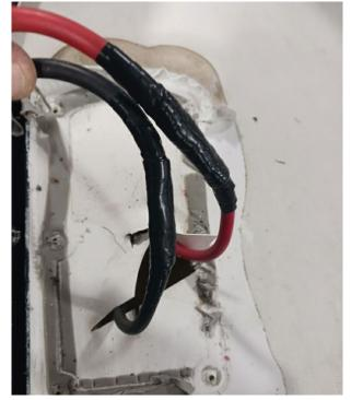
6. You will now reinstall the port, reconnect your input wiring from the solar panels and seal the port with the provided tube of self-leveling lap sealant.
