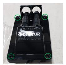
3. Remove fasteners and remove the port from roof. This will expose the wiring and the connection point we are looking for.
