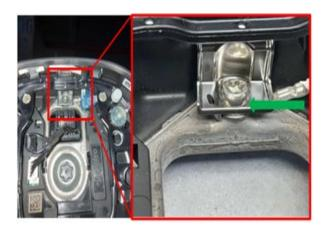
6. If the ground screw is in full contact with the horn plate bracket, check the torque of the screw using a torque wrench (2.5 Nm +- 0.5 Nm). Continue to Step 7 once completed.
