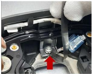
B. To help determine that there is no relative movement, use a 0.1 mm feeler gauge between the bottom of the screw head and horn pad bracket (lower arrow).
