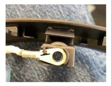
Note: DO NOT check the tight fit on the cable shoe of the ground strap. Be careful when inserting the screw, as the geometry of the cable shoe is sensitive to compressive and tensile loads.
