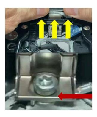
A. Press the horn cover from the inside out (upper arrows) to observe any possible movement of the horn plate bracket and screw.
