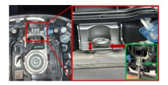
3. Using a magnifying glass, visually inspect the ground screw to determine if the screw is fully seated against the horn plate bracket.
