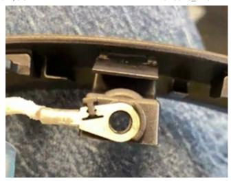
Be careful when inserting the screw, because the cable lug is sensitive to force and tensile loads due to it geometry.
