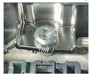
4. If the ground screw is NOT in contact with horn plate bracket, the screw must be removed, and the threads on the screw and in the steering wheel must be inspected for any burr formation.
