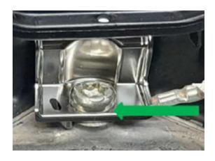
6. If the ground screw is in full contact with the horn plate bracket, check the torque of the screw using a torque wrench (2.5 Nm +- 0.5 Nm). Continue to Step 7 once completed.
