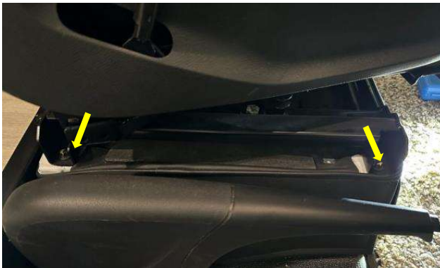
Image 2 – Seat attached to base.
