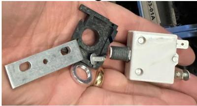
1. Locate the Winnebago 12v breaker panel under passenger's seat and remove the plug left of the 40a coach breaker – see Image 1, “Radio”. Install the new breaker panel label 358454-01-01a over the old label or trim the "Awning Chassis" and "Awning coach" out of the new label and place it over ""Awing – Toilet – Radio" to speed up the installation.
