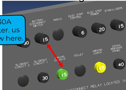
If the 30A slideout and 15A awning breakers are connected by a buss bar, **remove and discard Buss bar**. Add chassis power jumper from triple buss bar above to lower "Chassis awning" breaker connection and connect the original 8 Ga feed cable to the 30 A slideout breaker.
