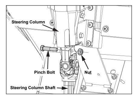
Figure 3, Steering Column Shaft
