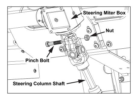
Figure 2, Steering Column Shaft
