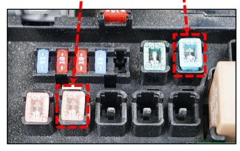
4. Adhere the new ESC1 <u>20A</u> and ESC2 <u>30A</u> labels to the bottom of the junction box fuse cover, as shown.
