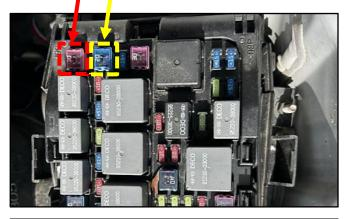
4. Adhere the new ABS1 <u>20A</u> and ABS2 <u>30A</u> labels to the bottom of the junction box fuse cover, as shown.
