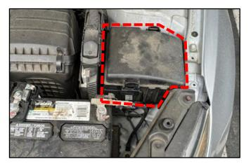
4. Disengage the clip and pull up to remove the bolt cover (A).
