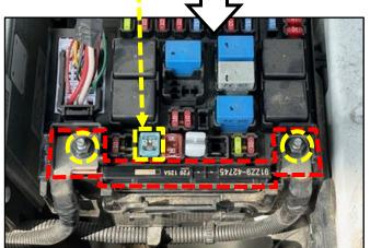
Note: Drill a hole through the center of the removed Multi Fuse. DO NOT reuse.
