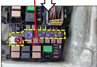
Note: Drill a hole through the center of the removed Multi Fuse. DO NOT reuse.
