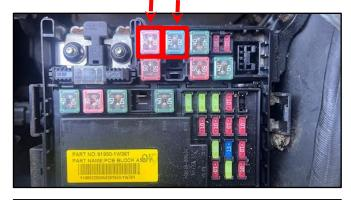
4. Adhere the new ABS1 <u>30A</u> and ABS2 <u>20A</u> labels to the bottom of the junction box fuse cover, as shown.
