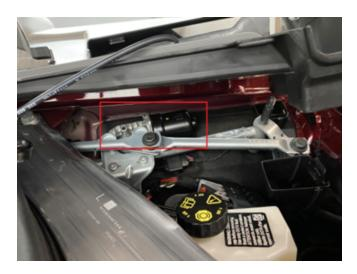
5. Raise the windshield panel cover on the driver side and record the wiper motor code.
