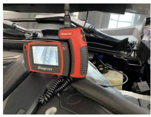
4. Remove the driver side wiper arm following the repair instructions "**Removing and installing/replacing both windshield wiper arms** 61 61 100 | REP-REP-P-6161100-G70 – V.1" (detach wiper arm with special tool **0 493 441 (61 6 060)** when necessary.)
