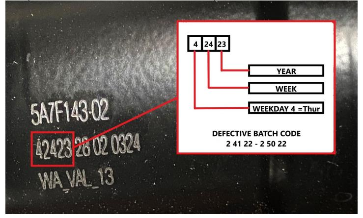
7. When the batch code falls under the affected dates (from **2 41 22** to **2 50 22**), the wiper linkage must be replaced. Refer to repair instructions "**Replace the console for the windshield wiper system** 61 61 271 | REP-REP-P-6161271-G70 - V.3" available with ISTA 4.40.5X.
