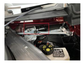
5. Raise the windshield panel cover on the driver side and record the wiper motor code.
