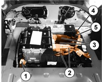
Check that the ground cable (1) is tightened to the prescribed torque of 15 Nm (11 Ft. Lbs.).
