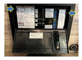
With the cover detached, remove the mounting screws to pull the power center from the cabinet.
