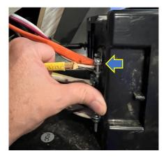
After the wire has been removed, retighten the wire clamp on the back of the power center.
