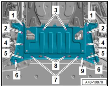
• Reinstall reinforcement and torque fasteners as follows:
