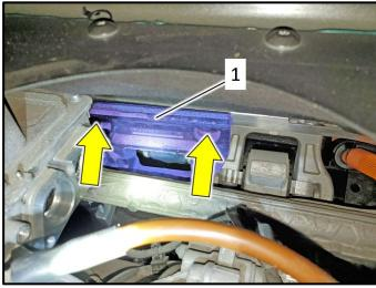
• Reinstall foam insert <1> and ensure securing pins <arrows> are fully engaged.
