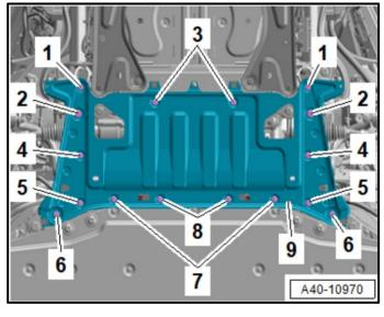
Reinstall reinforcement and torque fasteners as follows:
