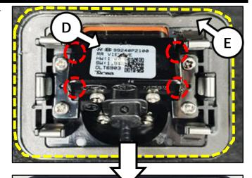
7. Replace the existing rear view camera mounting base (E) with the new mounting base E), RVM or SVM as applicble.
