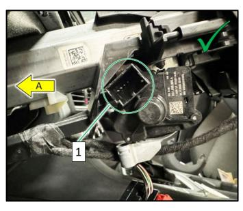
• The ignition switch is installed correctly, note the position of the connector housing <1> and the direction of travel <arrow A>.
