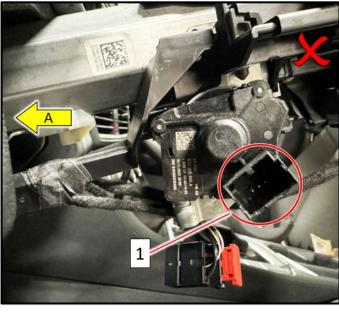
The ignition switch is not installed correctly, note the position of the connector housing <1> and the direction of travel <arrow A>.
