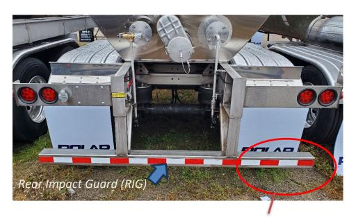
1) Tag will be installed on the passenger side of the RIG, on the *forward* side.
