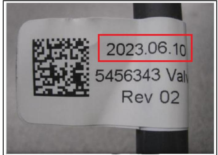
Verify the manufacture date is **NOT** within the range shown below. Fuel lines produced outside of the date range shown can be used for this recall.
