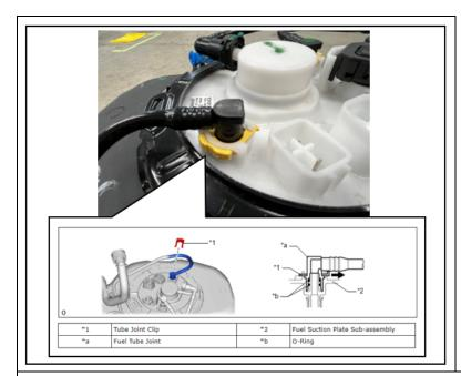
a. Align the fuel tube connector with the fuel pipe, push the fuel tube connector onto the fuel pipe, and then push in the retainer to secure the connection.
