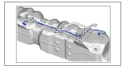
b. Remove the three clips securing the fuel tube to the fuel tank assembly.
