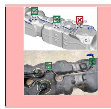
a. Align the fuel tube clip with the fuel pipe and push the fuel tube into the clip to secure it to the tank.
