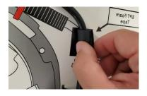
3. Once aligned, install the corrugated tubes in the 3 locations specified and apply electric tape to the fuel line according to the template. This tape should completely cover the corrugated tube. The tape should overlap onto the tube as it will secure the corrugated tube to the fuel tube.
