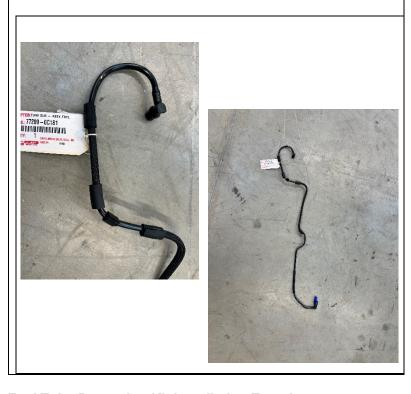
NOTE: If the fuel tube has been replaced previously it will already have corrugated tube applied. This tube will still require a repair kit. Please keep additional pieces from the kit and use them later if required. This vehicle will still need to come back for the remedy when available.
