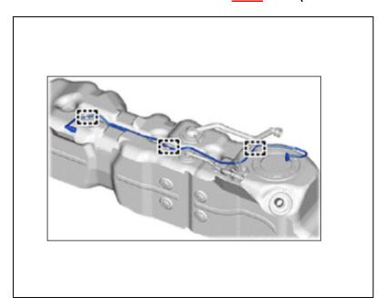
a. Remove the fuel tank to canister fuel hose.
