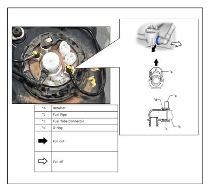
b. Remove the fuel tube connection at the fuel sending unit.
