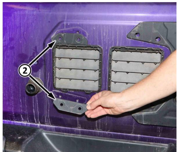
Figure 10 – Tire Carrier Mopar Hinge Reinforcement Bracket Spacers
