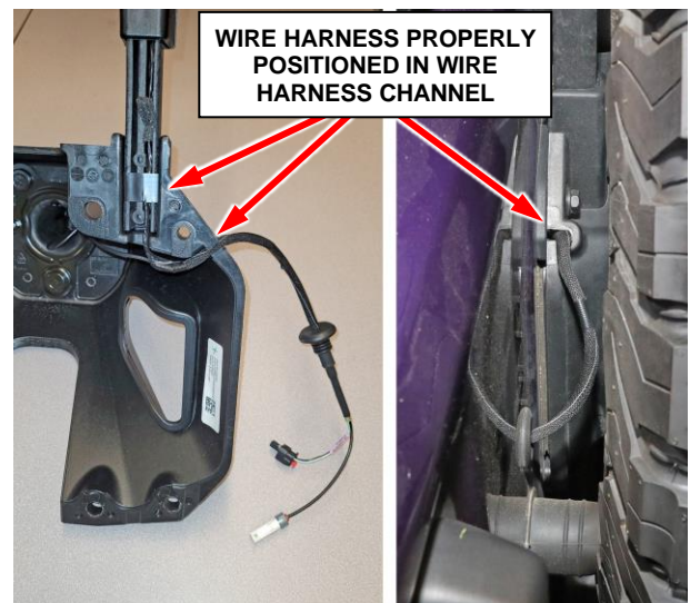
Figure 12 – Wire Harness Position
