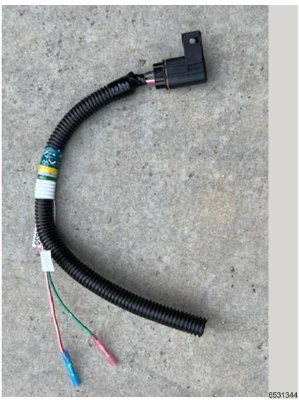
11. Crimp a red connector to the small wire and a blue connector onto the large wire of the replacement fuse harness.
