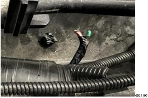
7. Cut the two wires to remove and discard the J-433 fuse holder (cut as close as possible to the fuse holder).
