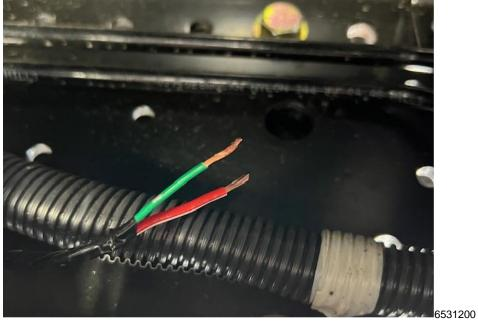
8. Remove the tape from the vehicle wires to expose about 25mm of wire. Strip about 7mm of insulation off the end of each wire. Confirm whether/that there is NO corrosion present. If there IS corrosion, cut the wire back further until you reach non-corroded material.
