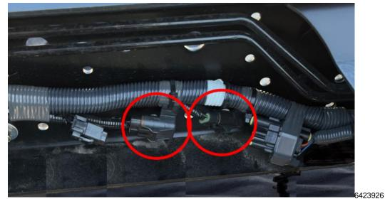
5. Locate the inline ignition fuse holders J-432 and J-433 (4500s shown on top, 5500s on bottom). Cut and remove the two zip ties and tape securing the fuse holders.
