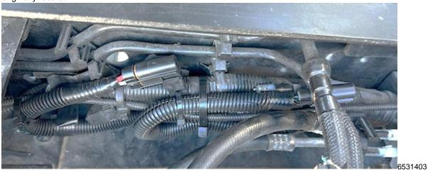
18. For 4500/4500HD only - Use wire ties to secure both replacement fuse conduits to the chassis harness.
