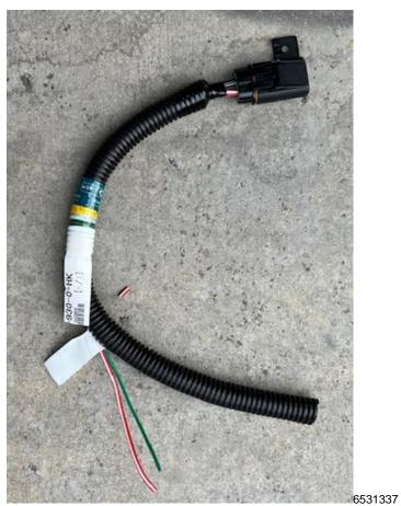
9. Partially remove the wires from the conduit on one of the replacement fuse holder harnesses.
