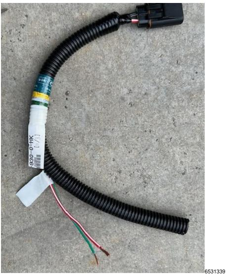
10. Strip about 7mm of insulation off the end of each of the wires of the replacement fuse harness.
