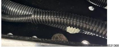
14. Push the wiring back into the replacement fuse harness conduit. Insert the small vehicle conduit into the larger replacement fuse harness conduit.
