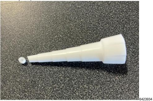
9. Prepare the SuperX Silicone by cutting the very tip of the applicator nozzle off.
