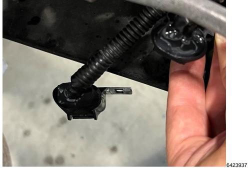
11. After ensuring each wire is covered where it exits the connector, fill the remaining area of the cup with silicone.
