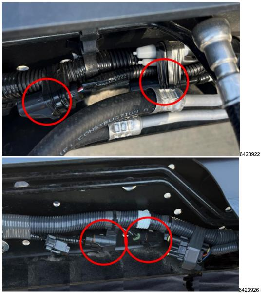
5. Locate the inline ignition fuse holders J-432 and J-433 (4500s shown on top, 5500s on bottom). Cut and remove the two zip ties and tape securing the fuse holders.
