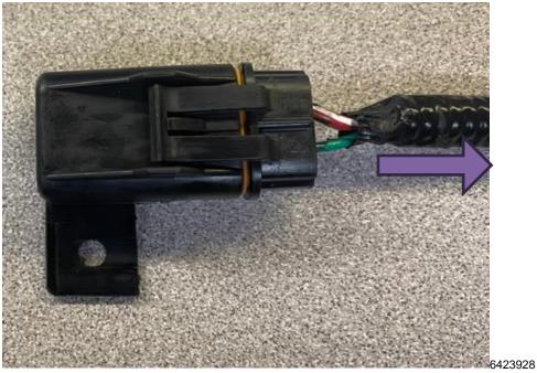
6. Gently pull the corrugated tube and PVC tape away from the fuse holder.
