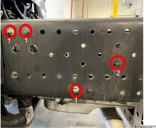
2. (For 4500/4500HG ONLY) Remove three nuts & bolts (indicated by 1 above) securing the transmission cooler lines and release one (indicated by 2 above) chassis harness clip.
