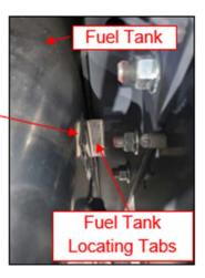
**14.** Install the 3 fuel tank straps in the correct location as shown. For each of the 3 upper fuel tank strap mounting locations, install the clevis pin, washer and cotter pin.
