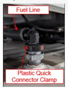
**18.** Connect the fuel supply hose, fuel return hose to their corresponding fuel tank fittings and then position the spring clamps back to their original installed positions.
