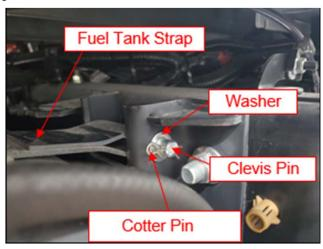
10. Remove the fuel tank from the vehicle.
