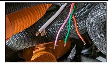
6. Join the selected wire and match it to the vehicles wiring harness, as shown.
