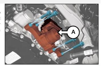
1b. Note: Place a container under the vehicle to drain any residual oil when removing the EOP assembly. Take note of the amount drained as the will need to be refilled during reassembly.
