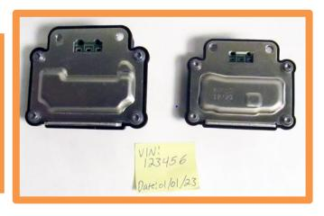
8. Confirm the orange seal is correctly in place on the EOP.
