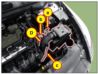
4. Disconnect the ETC module connector (E).
