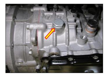
17. Allow the IVT fluid to flow out until it flows in a thin steady stream. If necessary, add additional IVT fluid until it flows in a thin steady stream.
