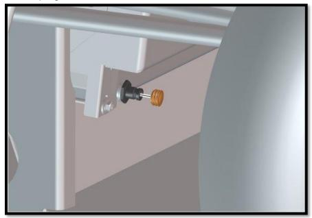
8. Drain the cooling system using either a coolant extractor or a drain hose and pan.
