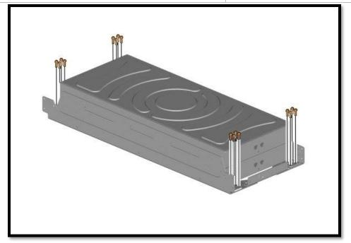
88. Remove the nuts and the screws.
