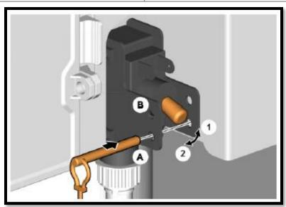
158. Disconnect the rear coolant pump.
