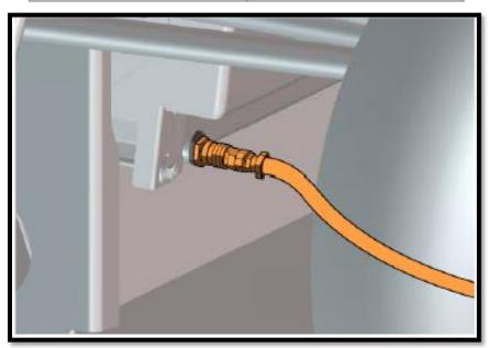
158. Loosen the bleeder screws.
