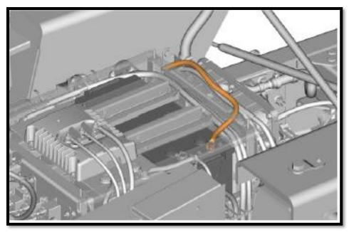
163. Unlock the negative terminal along with the fuses.
