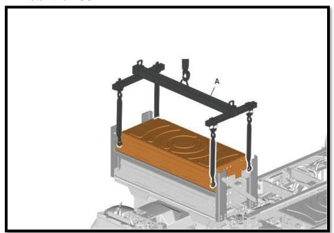
137. Remove the lifting tool.
