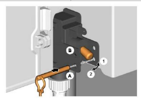
158. Disconnect the low voltage ESS connectors.
