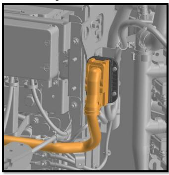
160. On MPB side of the cooling box interface connector, jump **Pin 56** to **Pin 54** and
