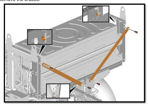
45. Remove the nuts and the screws.
