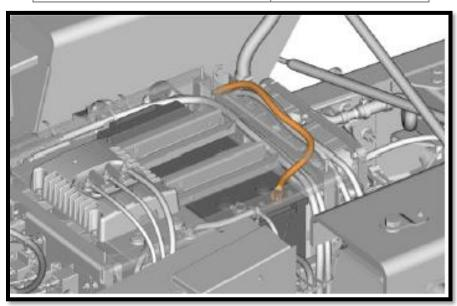
159. Install the fuses. Install the nuts. Torque tighten the nuts.
