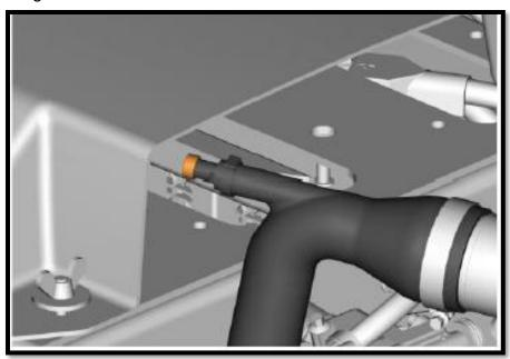
168. Check the coolant level. Adjust as necessary
