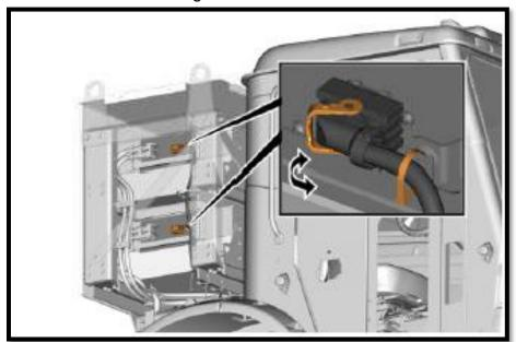
163. Remove the safety pin from the slot (B) and install in slot (A). Set the chassis switch to position (2).
