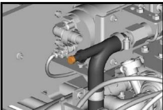
163. Reconnect the coolant pumps. Remove the jumper and connect the connector.
