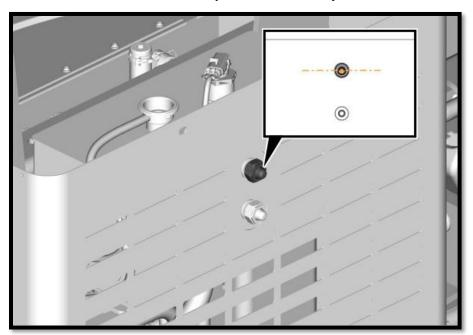
169. Remove the safety pin from the slot (**A**) and install in slot (**B**). Set the chassis switch to position (**1**)
