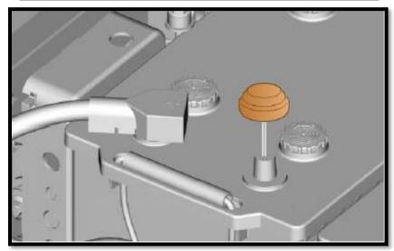
158. Connect the cable to the negative terminal. Torque tighten the nut.
