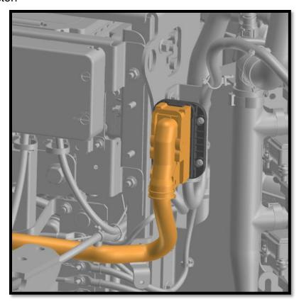
164. Connect the rear coolant pump.
