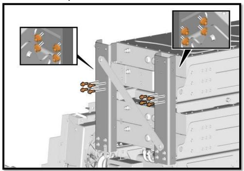
94. Remove the nuts and the screws.
