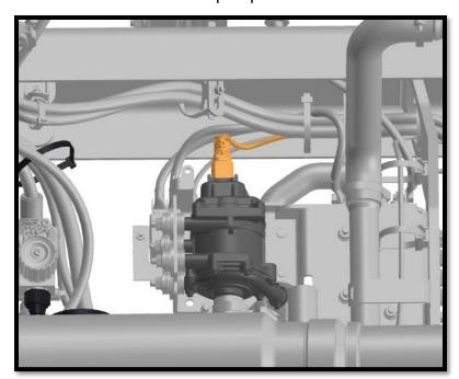
159. Disconnect the cooling box connector.
