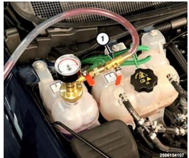
Figure 73 – Cooling System Refill
