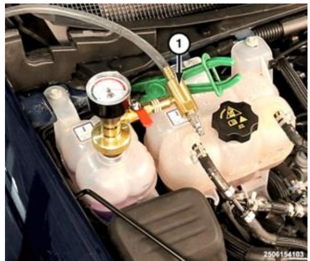
Figure 69 – Cooling System Refill
