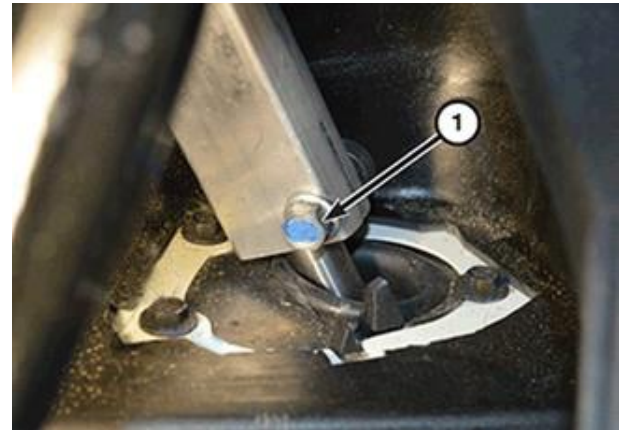
Figure 26 – Steering Gear Pinch Bolt
