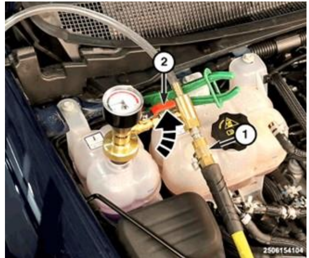
Figure 70 – Cooling System Refill
