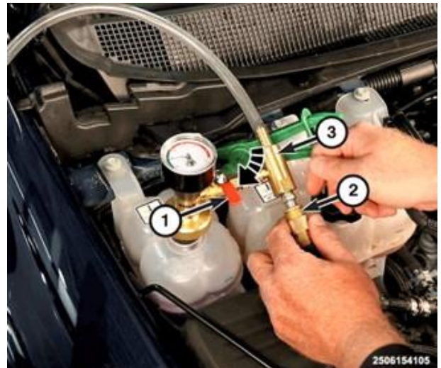
Figure 71 – Cooling System Refill
