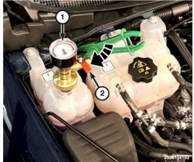
Figure 68 – Cooling System Refill
