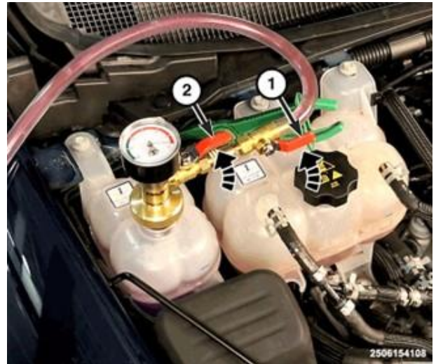
Figure 74 – Cooling System Refill
