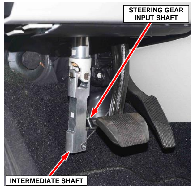
Figure 27 – Steering Gear Pinch Bolt
