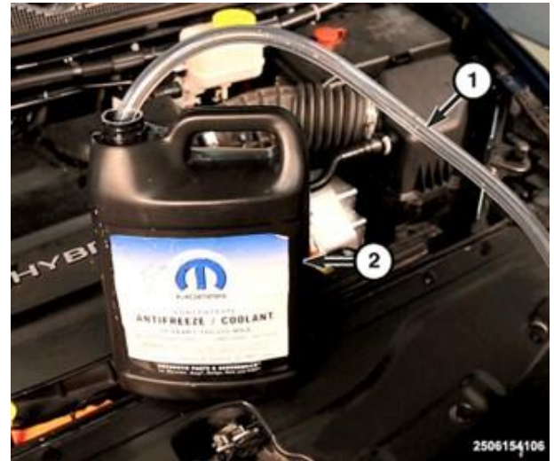
Figure 72 – Cooling System Refill
