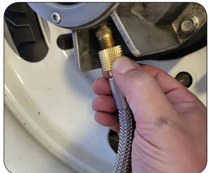
6. New tire hose assemblies can be identified by the yellow spiral wrap around the stainless steel braid (**Figure 18**). Make sure the hubcap to rim clcking is correct to be able to assemble the hoses in Step 5. If the trailer has had tires serviced, these could be incorrect.
