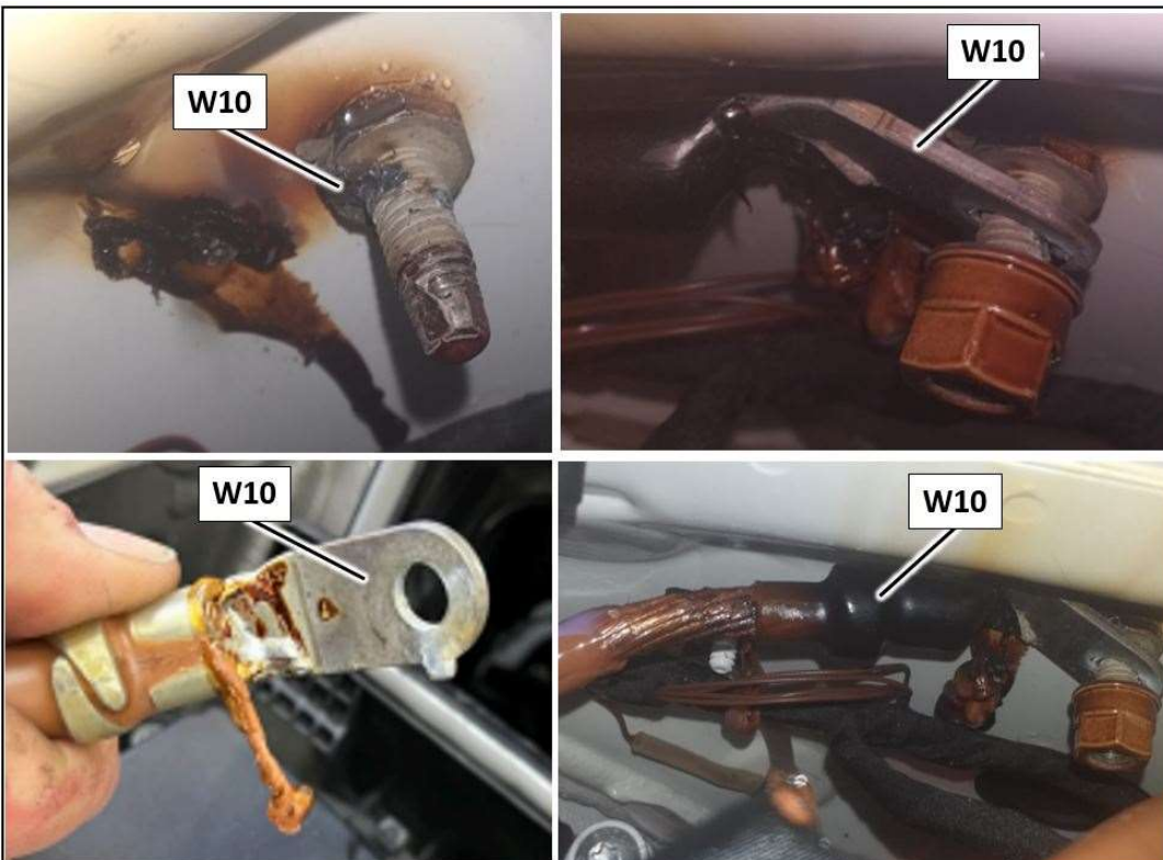
Figure 6, Examples of potential damage profiles of an on-board electrical system battery ground point (W10)
