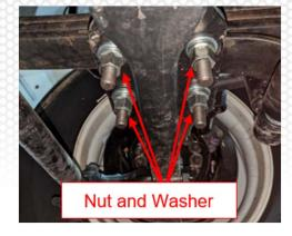
**5.** Tighten all four driver side front U-bolt nuts to the specified torque. Follow the tightening sequence for each side called out in the diagram to the right.
