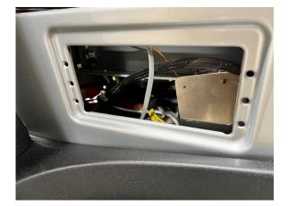
2. Under the pedestal, looking to the left, inspect the fuse block/terminal for a blue colored fuse. A blue fuse represents 200A, which would need replaced by a 50A fuse. If the color of the fuse is red, this represent a 50A fuse, which is the correct size. No further action is required if a 50A fuse has been installed.
