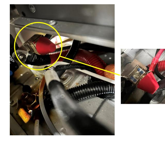
3. If a 200A fuse has been installed, begin by unscrewing the four E12 bolts from the driver's seat.
