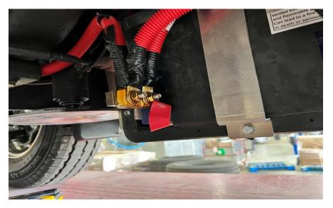
13. Finally, reinstall the battery cover using the four 3/8 self-tappers and a 3/8 socket.
