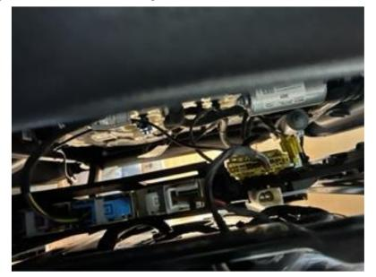
5. To disconnect all power to the unit to service the fuse, locate the house battery installed under the passenger side step well. A 3/8 nut driver will be required to remove the four self-tapping screws securing the battery cover.
