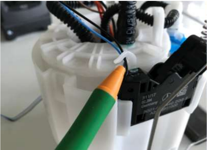
Figure 4 (remove lines from routing clip)
