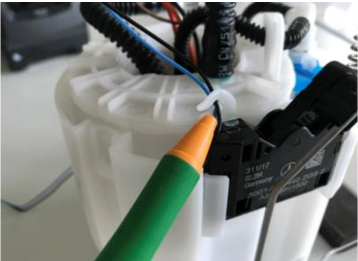
Figure 4 (remove lines from routing clip)
