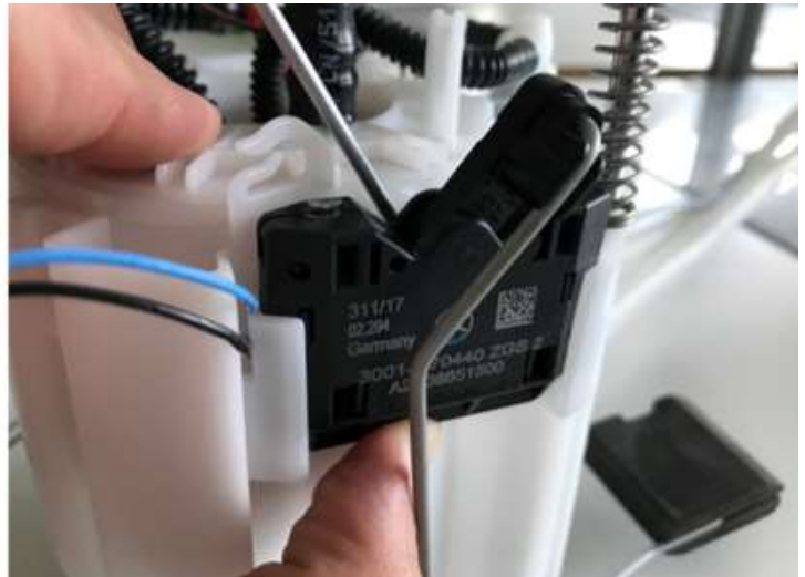
Figure 5 (using a screwdriver, carefully push float-and-lever sensor housing away from module housing and at the same time push float-and-lever sensor housing upwards.)
