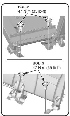
19. Remove the third-row lower seat cushion by removing the three bolts.
