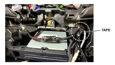
40. Tape the 90 deg splice boxes and FAKRA Splice repair service cable harness to the dash harness.
