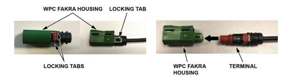
2. Release the lock tab and remove the terminal from the vehicle harness.
