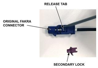
3. Pull to remove the housing from the cable and then discard the housing and secondary lock tab from the FAKRA splice repair service cable.
