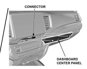
10. Remove the screws and bolts to remove the Blu-Ray player or dashboard center lower panel.
