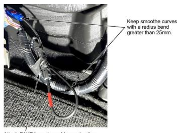
Attach FAKRA service cables and splice boxes to the appropriate component harness with tape to prevent any rattles.
