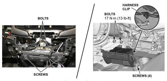
11. Loosen the two bolts holding the Infotainment Control Unit and then, remove the unit.
