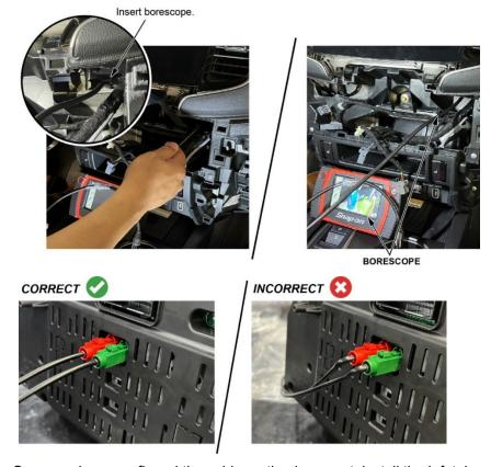
8. Once you have confirmed the cable routing is correct, install the Infotainment Control Unit mounting screws.
