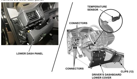
4. Pull back the dash panel to allow meter bezel removal.
