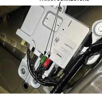
2. Install the matching color FAKRA splice repair service cables and splice box.
