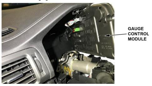
2. Disconnect the red and green FAKRA connectors and any other related connectors from the gauge control module.
