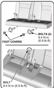
21. Remove the two front bolts for the passenger third-row seat back.
