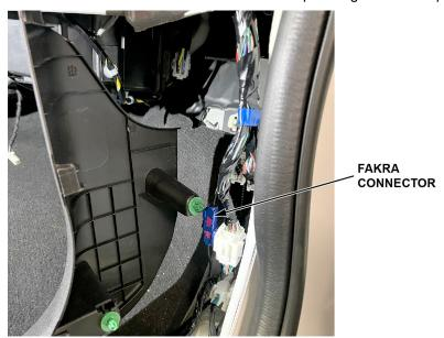
2. Install the matching color FAKRA splice repair service cable and splice box.
