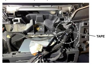
18. Tape the FAKRA splice repair service cable harness to the dash harness.
