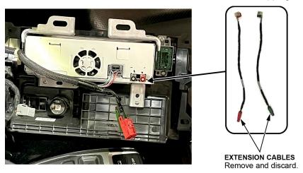
4. Install the matching color 90° FAKRA splice repair service cables and splice boxes.
