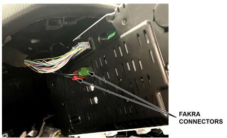
3. **If** the WPC FAKRA service housings and extension cables are installed, un-tape the WPC connectors, and extension cables from the vehicle harness.
