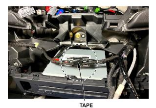
41. Using the digital borescope (T/N BK5600DUAL55) or a commercially available borescope with multiple view angles, inspect the cable routing at the back of the gauge control module as shown below to make sure the cables are routed straight and not sideloaded. Adjust gauge control module harness as needed to achieve proper cable routing.
