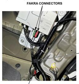
Attach the FAKRA service cables and splice boxes to the appropriate component harness with tape to prevent any rattles.
