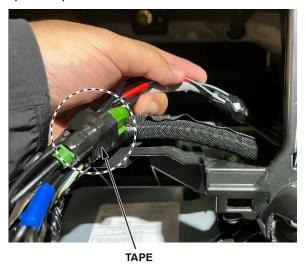
17. Tape the FAKRA splice repair service cable harness to the vehicle harness at the lower dash.
