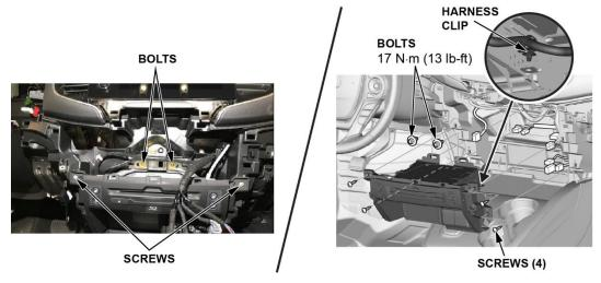
11. Loosen the two bolts holding the Infotainment Control Unit.
