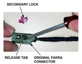
2. Pull to remove the housing from the vehicle harness. Then, **discard** the housing and lock.
