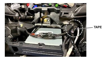
40. Tape the 90 deg splice boxes and FAKRA Splice repair service cable harness to the dash harness.
