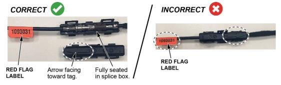
8. Once the FAKRA splice repair service cables and splice boxes have been attached to the cable connection, tape the splice boxes and FAKRA service cables to the appropriate component harness.
