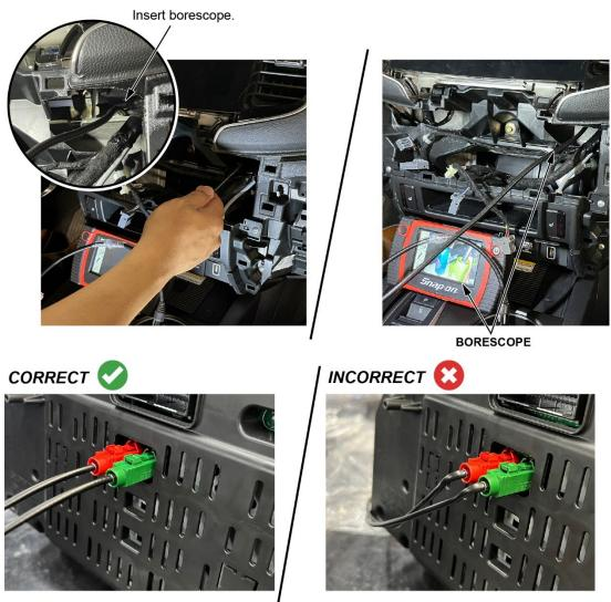
42. Once you have confirmed the cable routing is correct, install the Infotainment Control Unit mounting screws.
