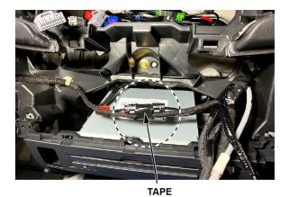
41. Using the digital borescope (T/N BK5600DUAL55) or a commercially available borescope with multiple view angles, inspect the cable routing at the back of the gauge control module as shown below to make sure the cables are routed straight and not sideloaded. Adjust gauge control module harness as needed to achieve proper cable routing.
