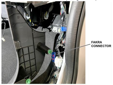
2. Install the matching color FAKRA splice repair service cables and splice box.
