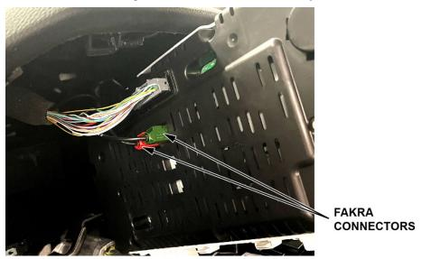
3. **If** the WPC FAKRA service housings and extension cables are installed, you must un-tape the WPC connectors and extension cables from the vehicle harness.
