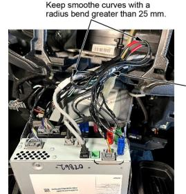
Attach FAKRA service cables and splice boxes to the appropriate component harness with tape to prevent any rattles.
