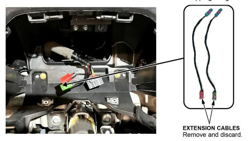
5. Install the matching color FAKRA splice repair service cables and splice boxes.
