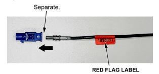
4. Connect the appropriate color FAKRA splice repair service cable to the vehicle harness.
