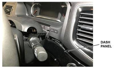
5. Remove the meter bezel and upper column cover as one piece.
