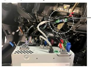
Tape both splice boxes, green connector and cables to the infotainment control unit.
