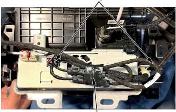
Attach FAKRA service cables and splice boxes to the appropriate component harness with tape to prevent any rattles.
