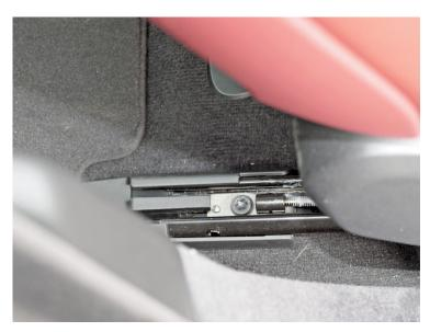
Inspect the right rear of both front seat rails for insufficient welding.
