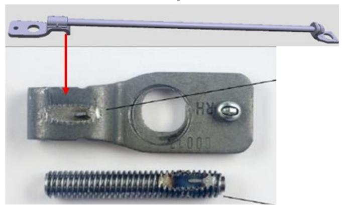
Inspect the seat rail closely and read the batch number. If the mounting bolt is in the way of reading the batch number, it can be removed but must be replaced even if the seat rail is not being replaced.
