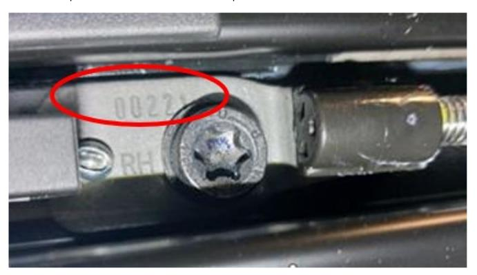
**NOTE**: When replacing the seat rail, follow Repair Instruction **REP 52 14 010** (Removing and mounting/replacing both seat rails on front seat at left or right) and make sure to transfer any installed end stop that is on the rail or the seat module will fail to initialize after installation of the new seat rail. Reference Copyright ©2023 BMW of North America, Inc.
