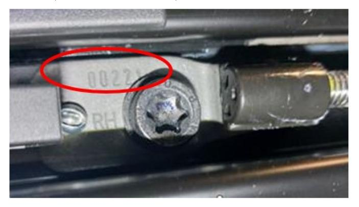
**NOTE**: When replacing the seat rail, make sure to transfer any installed end stop that is on the rail or the seat module will fail to initialize after installation of the new seat rail. Reference SI B52 01 21 about seat rail end stops.
