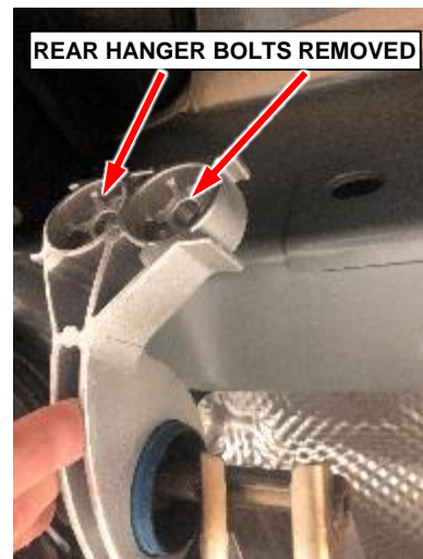
Figure 5 – Rear Exhaust Hangers
