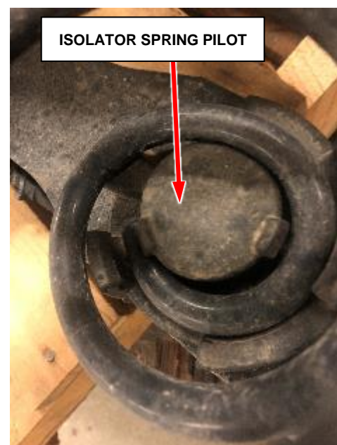
Figure 2 – Coil NOT On Top of the Isolator Spring Pilot
